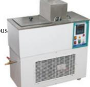
Features :a) Temperature Range :-30 to 90 °Cb) Digital Temperature controller accuracy +/- 0.5 °C.
